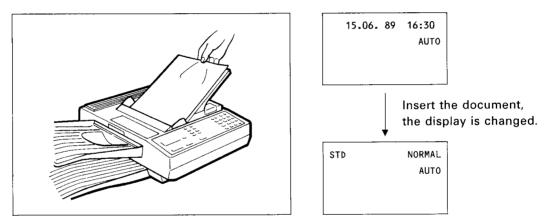
You can load up to 20 sheets in the automatic document feeder. Stagger the leading edges of the sheet slightly, and insert the sheets with a slight push to assure smooth feeding.
